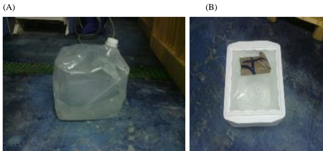
Figure 7.5.1. (A) 20 l cubitainer and (B) Styrofoam box with ice pack in cardboard, used for the shipping of fish eggs.
