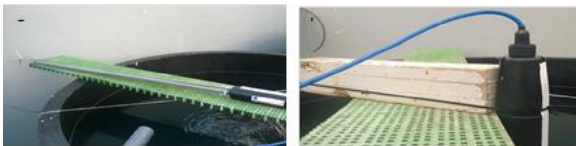
Figure 15.3.1.2 The holding construction of the velocimeter on the top of the tank (a) and detail of the positioning of the sensor (b)
