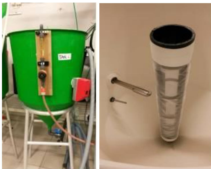
Figure 17.3.1. Artemia tank showing water supply and outlet sieve.
