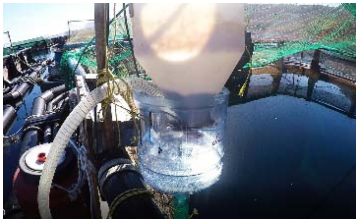
Figure 20.3.3.2. Feeder installed during the trial for the submerged feeding
