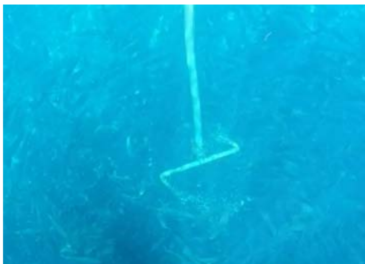
Figure 20.3.3.3. The S-form ending of the submerged feeding system
