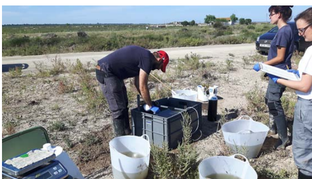
Figure 23.4.2. Set-up for the field sampling including extra oxygen supply.
