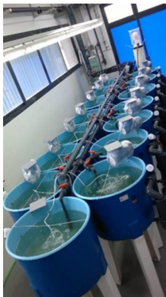
Figure 23.4.1 RAS system used to acclimatize and grow the grey mullet fingerlings before seeding in the farm ponds.
