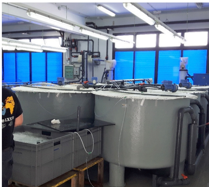
Figure 13.10. RAS system used for the trial with the adult grey mullet at CTAQUA facilities.
