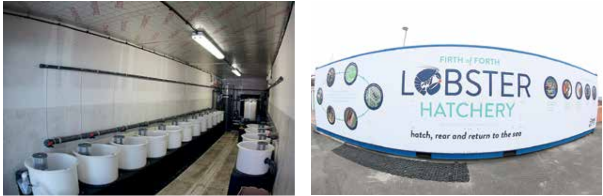
Figure 8.9. Hatchery in a box, containing larval rearing vessels, Aquahive and RAS technology, incorporated and deployed inside a shipping container. (Images courtesy of Jane McMinn, Firth of Forth Lobster Hatchery)
