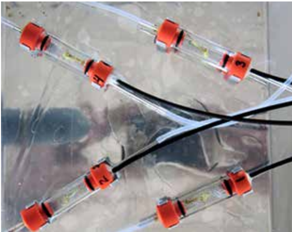
Figure 6. Intermittent flow respiration chambers for measuring oxygen consumption in zoea IV lobster juveniles. (Image courtesy of Ivar Lund, DTU Aqua.)
