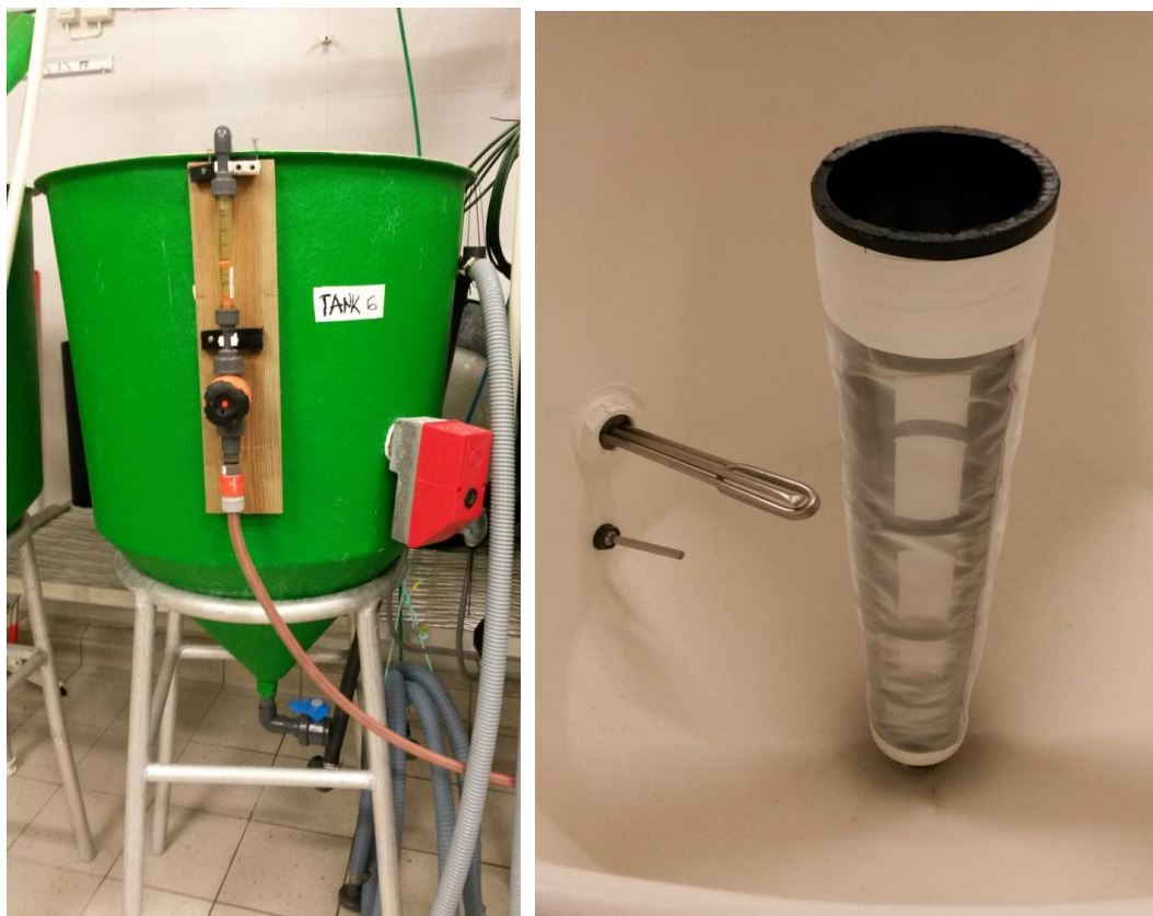
Figure 1. Artemia tank and outlet sieve.
