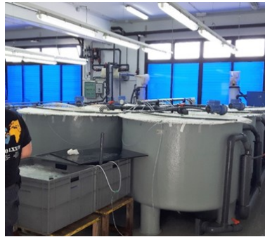
Figure 13.3.5.1. RAS system used for the trial with the adult grey mullet at Ctaqua facilities.
