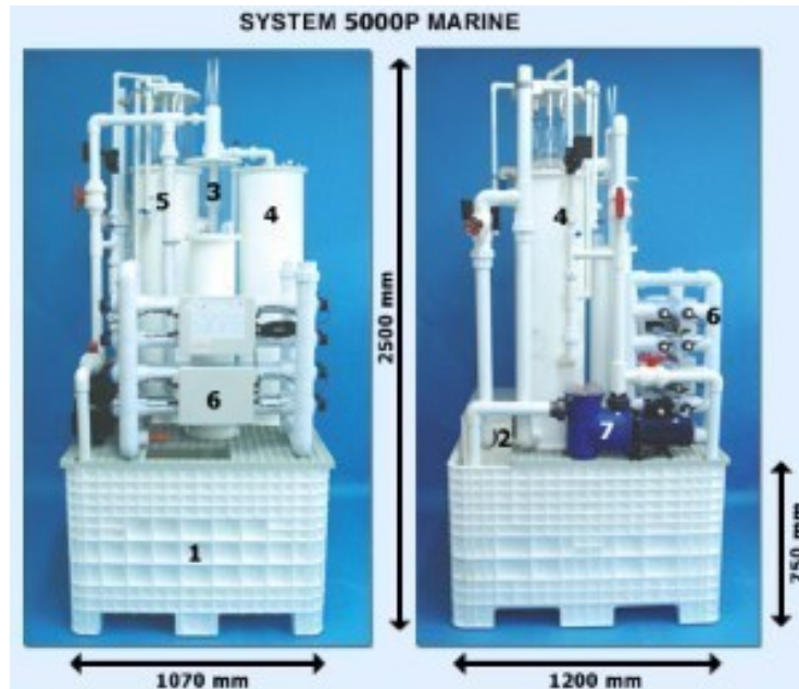
Figure 3. The RAS system P5000P MARINE from Tropical Marine Centre. The system consists of a reservoir (650 l), filter bags, sand filter, re-gassing / trickling biofilter and a protein skimmer.
