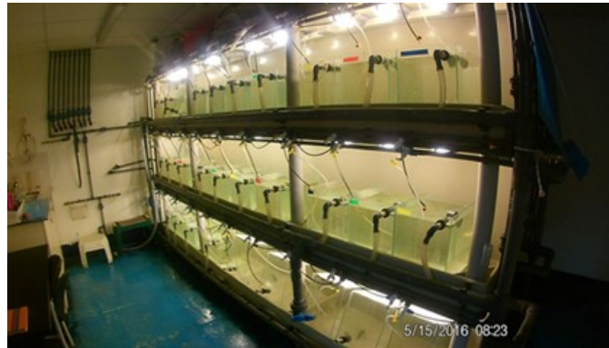
Figure 4 One side the sixty 17 l aquaria system with computer controlled salinity and temperature.
