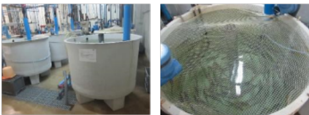
Picture 2.5.1.1. Experimental set up with six tanks connected in pairs to a recirculating aquaculture system (RAS, IRTAmor). Each pair of tanks were a programmed feeding regimen (Prog) and a auto-demand feeding system (AD).
