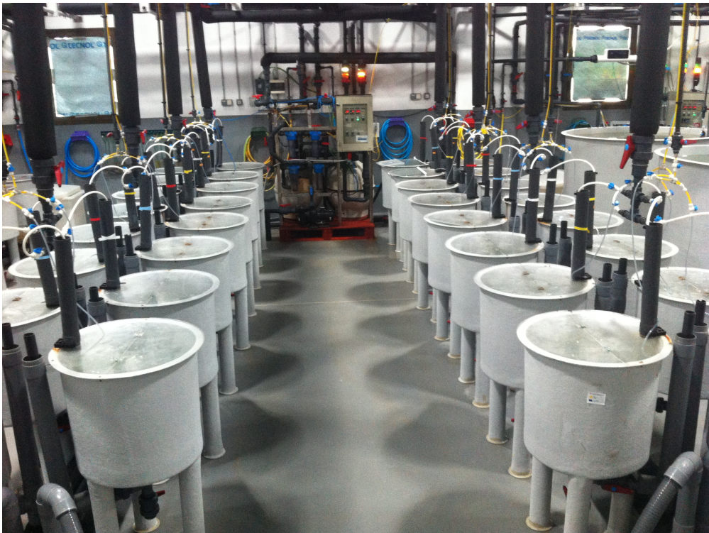
Figure 2. Experimental set up using IRTAmar ® RAS for meagre challenge with Vibrio anguillarum .
