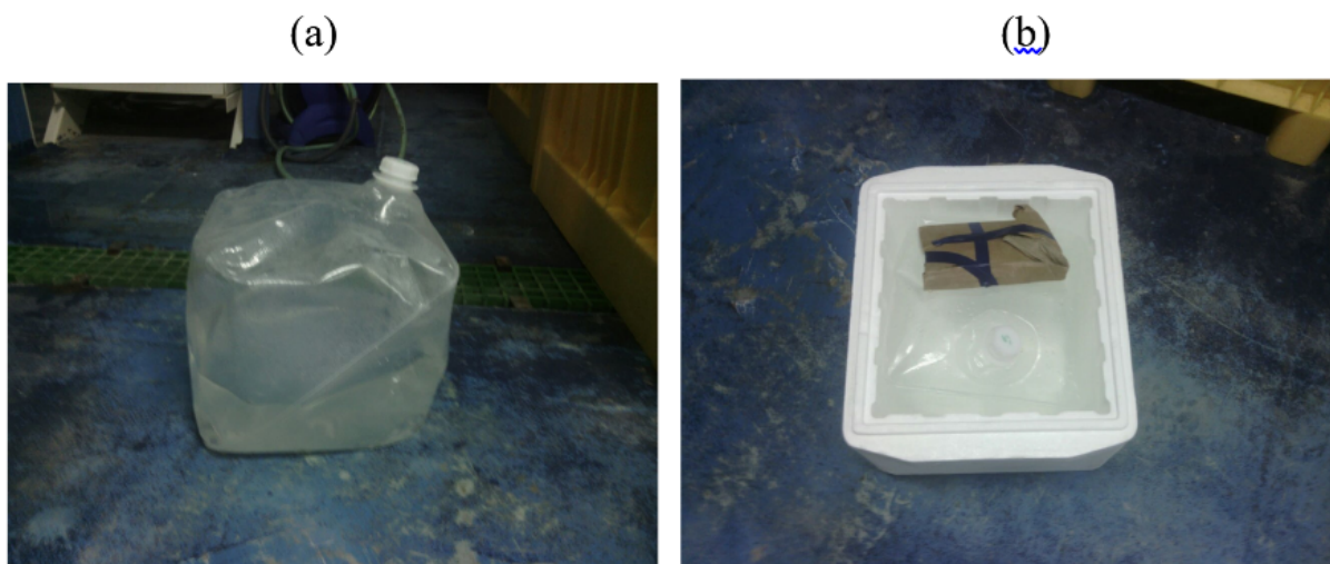
Figure 1. (a) 20 l cubitainer and (b) Styrofoam box with ice pack in cardboard used in the past to transport Atlantic bluefin tuna eggs and used in this study with grey mullet eggs.
