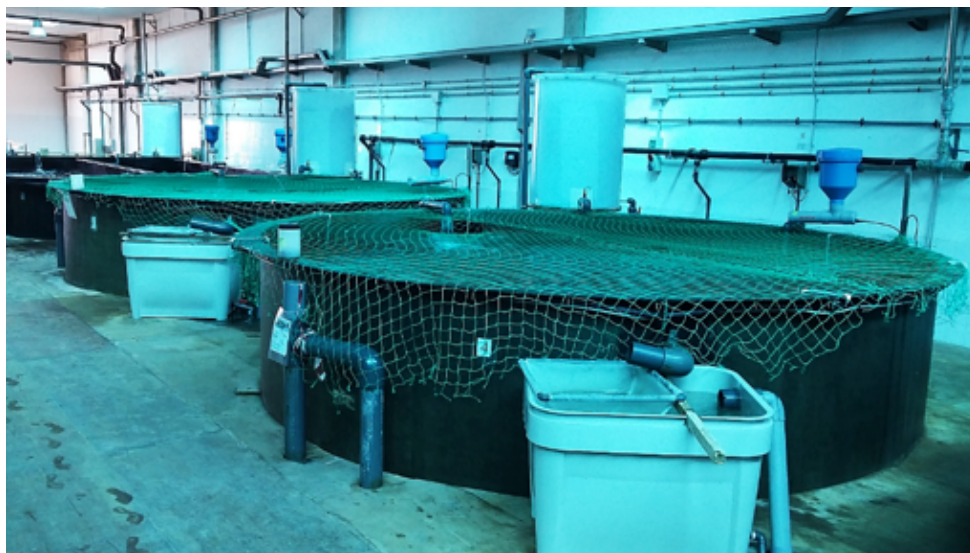
Figure 9.4.3. Experimental tanks of 40 m 3 (5 m x 2.35 m depth) at the facilities of the Grupo de Investigación en Acuicultura (GIA), located in the Parque Científico Tecnológico Marino (PCTM), of the Universidad de Las Palmas de Gran Canaria (ULPGC).
