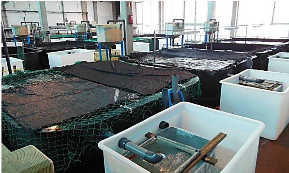
Figure 9.4.2. Experimental tanks of 10 m 3 (3 m x 3 m x 1.5 m depth) at the facilities of the Grupo de Investigación en Acuicultura (GIA), located in the Parque Científico Tecnológico Marino (PCTM), of the Universidad de Las Palmas de Gran Canaria (ULPGC).
