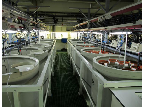
Figure 3 Experimental system of 18 1.5 m 3 tanks at the IOLR.
