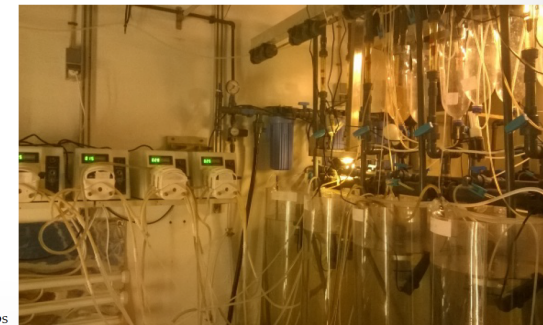
Fig. 1 Exp. setup, tanks and peristaltic pumps for accurate seawater flow
