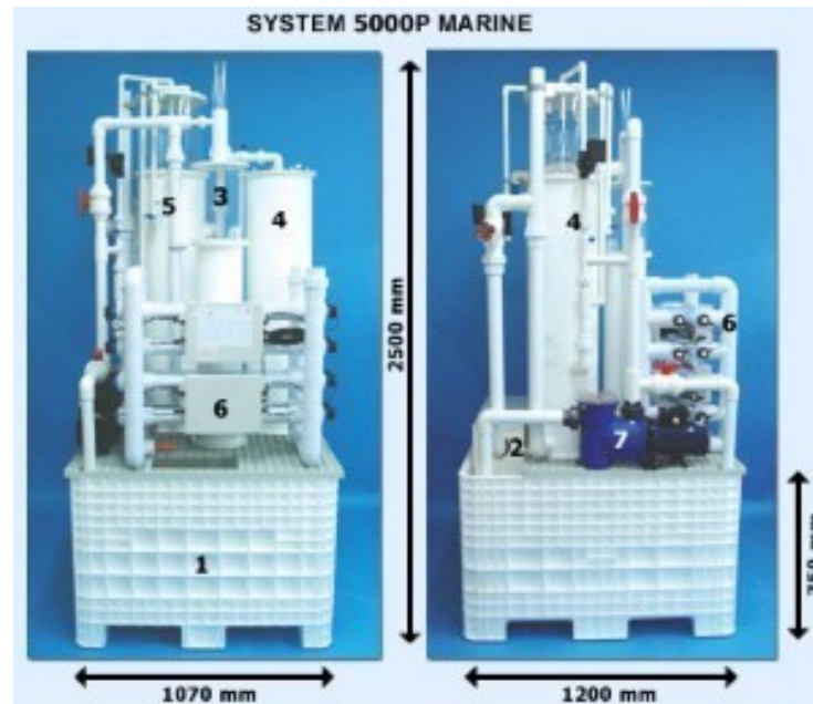
Figure 23. RAS system P5000P MARINE from Tropical Marine Centre. The system consists of a reservoir (650 liter), filter bags, sand filter, re-gassing / trickling biofilter and a protein skimmer.
