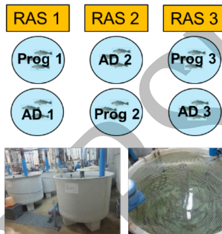
Figure 50. Experimental set up with six tanks connected in pairs to RAS, IRTamar. Each pair of tanks was a programmed feeding regimen (Prog) and a auto-demand feeding system (AD).
