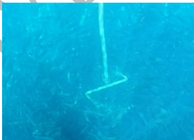
Figure 47. The S-form ending of the submerged feeding system
