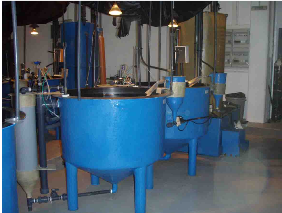
Figure 15.2.3 Larval RAS rearing tanks in P1. HCMR.
