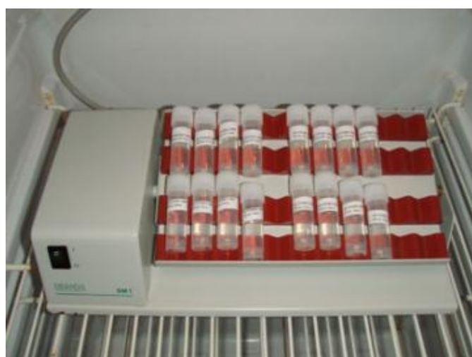
Figure 5.2.1 Set up for the in vitro release assay for the GnRH a implants (left). Mean (±SEM) GnRH a released from the GnRH a implants at 24°C (right).
