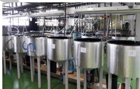
Figure 28. Cylindrical tanks for larval rearing experiments under different water temperatures.
