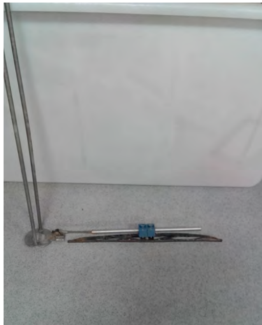
Figure 2. Automatic tank cleaning system at the bottom of the first feeding tank for Atlantic halibut larvae
